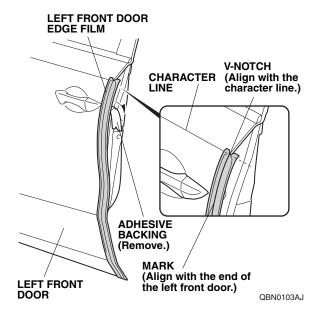
Align the mark on the left front door edge film with the end of the left front door. While applying light pressure, carefully remove the adhesive backing, and attach the left front door edge film to the left front door. Go to step 11.
