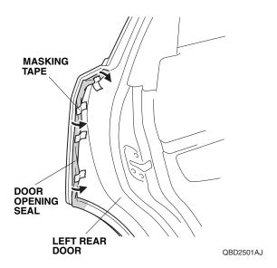
3. Using an alcohol swab, thoroughly clean the area where the left rear door edge film will attach.
