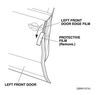
13. Starting from the center and working outward, use your fingers to fold the left front door edge film around the edge of the left front door. Move your fingers in one direction. Attach the left front door edge film over the seam sealant. Do not trim or damage the seam sealant.
