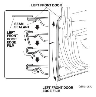
14. Using a shop towel, wipe the 3M protective tape application solution from the left front door edge film. Allow the left front door edge film to dry thoroughly.
