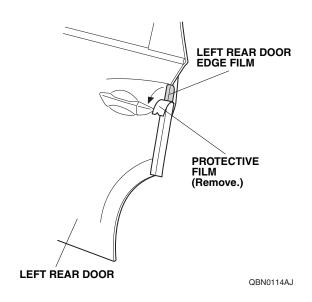
20. Starting from the center and working outward, use your fingers to fold the left rear door edge film around the edge of the left rear door. Move your fingers in one direction. Attach the left rear door edge film over the seam sealant. Do not trim or damage the seam sealant.
