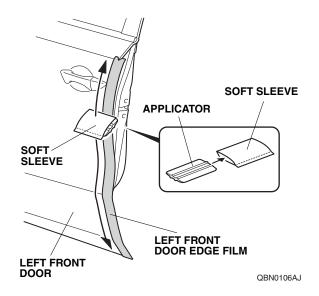
12. Slowly remove the protective film from the left front door edge film.
